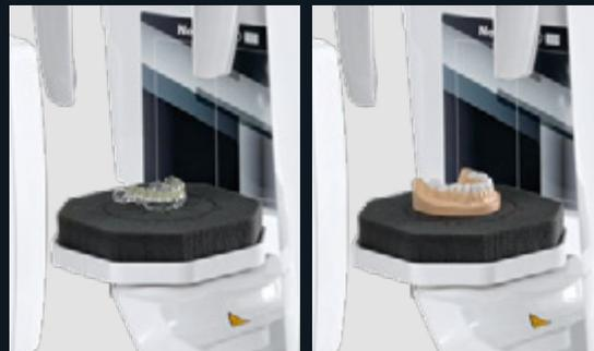
A specific protocol allows for tomographic scans of radiological templates, prostheses, models or impressions after they have been positioned on a special support.
